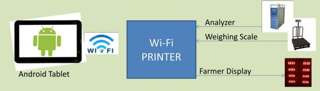
VERTEX TAB DPU is an Android TAB based solution for Milk collection centers. The tablet connects to a Wi-fi Printer also has serial interface ports to all common analyzers and weighing scales. The FAT/SNF information collected from the analyzer and weight from the scale are sent to the Tablet. It also drives a farmer display.
